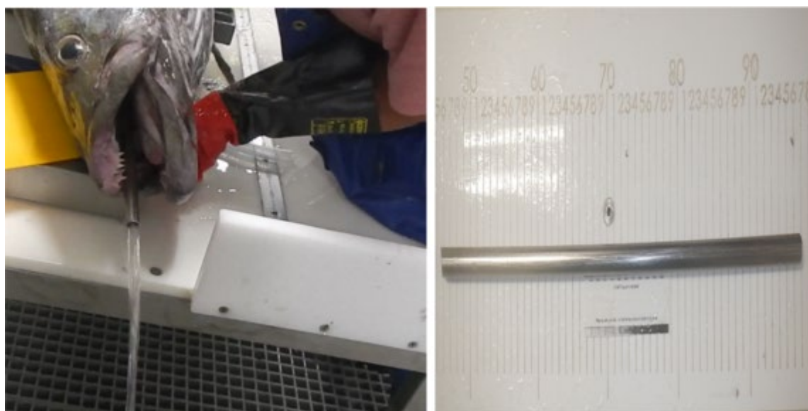
Figure 1: Demonstration of a drain tube used for draining toothfish stomachs of water.
