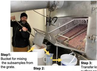
Fill two graduated measuring jugs with krill to the ~ 200ml mark and the ~ 50-100ml mark, respectively. Measuring cup with a subsample of ~ 200 krill
