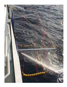
Figure 3: Bird Excluder Device used on the FV Janas.
